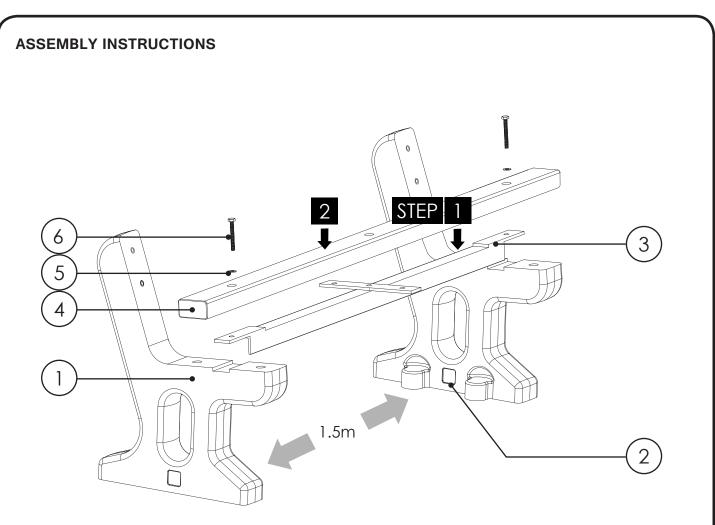
Stand Items 1 and 2 upright spaced approximately 1.5m apart with the base fixing lugs facing inwards (as shown). Slot Item 3 on top of both Seat Ends. The Support Brace locates into indentations in the tops of the Seat Ends. Take care to ensure the holes in the Support Brace align with the fixing holes in the Seat Ends and that the Support Brace is facing forwards as shown.
