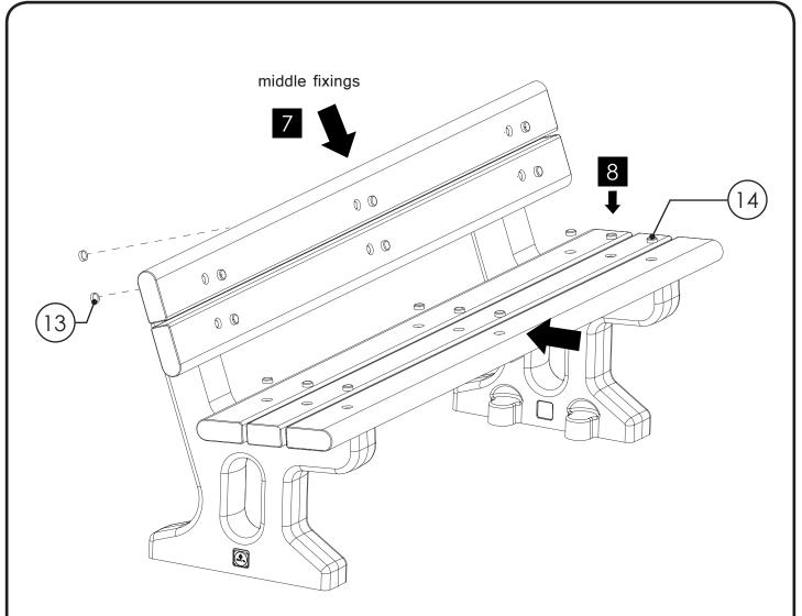
Tighten the middle set of five fixings first using the pair of sockets (or socket and spanner) ensuring the Slats are evenly spaced as you do so. Take care not to overtighten the middle pair of fixings in the Backrest as this may cause damage to the plastic Cover Caps. Then tighten the fixings attaching the Seat Ends to the Slats again ensuring the slats are evenly spaced before tightening fully.
