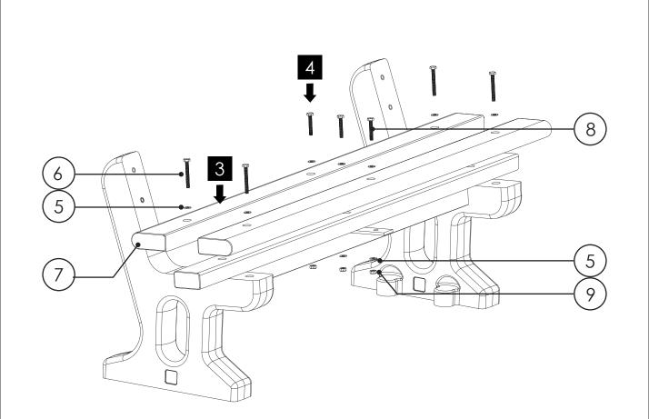
Place 2 x Item 7's onto the Seat Ends either side of the Slat fitted during STEP 2 with one of the 'bullnosed' ends facing forwards and other facing backwards (as shown). Assemble 4 x fixings by placing Item 5 onto Item 6. Place the fixings through the fixing holes in the Bullnose Slats and tighten the fixings loosely by hand.
