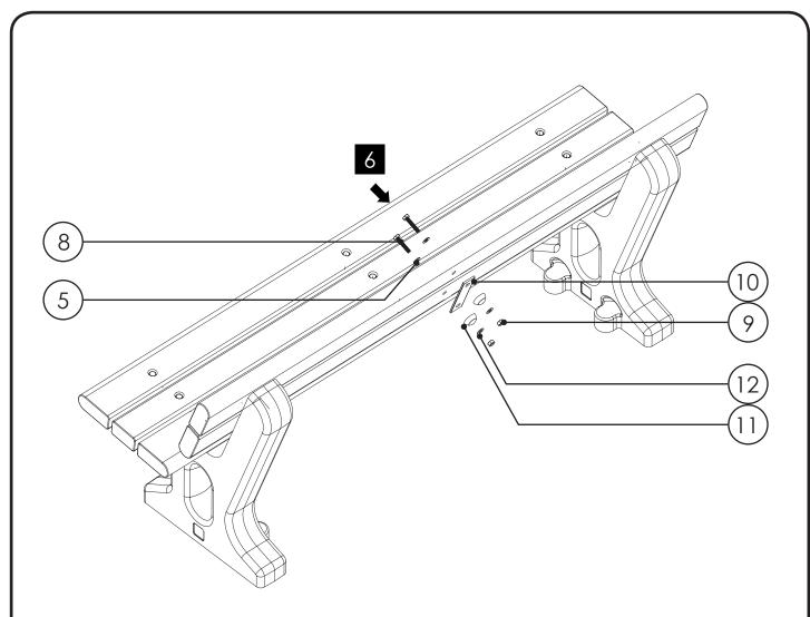
Assemble 2 x 60mm fixings by placing 2 x Item 5's onto Item 8's. Place the fixings through the middle fixing holes of the 2 x backrest Slats. On the back side of the Slats fit Item 10 over the fixing threads followed by 2 x Item 11's. Secure the fixings in place by adding Item 11 followed by Item 9 onto the screw threads. Loosely tighten the nuts by hand.
