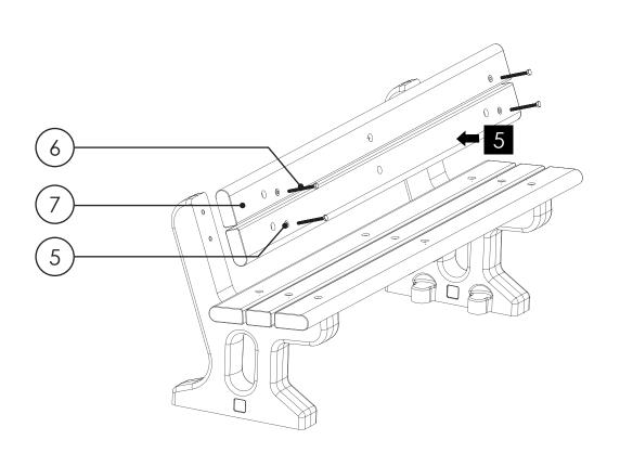
Assemble 4 x fixings by placing Item 5's onto Item 6's.
